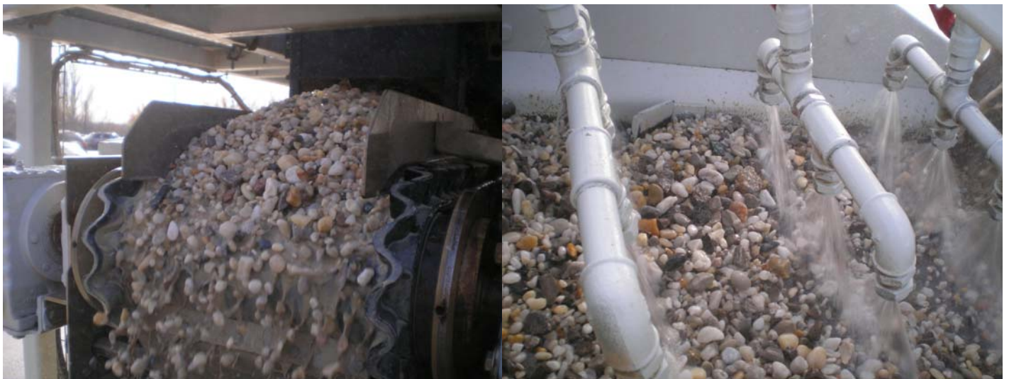
Figure 4 – Dis-agglomerated material exiting the Washing Chamber and entering the final rinse stage on a TYCAN Horizontal Vibrating Screen
