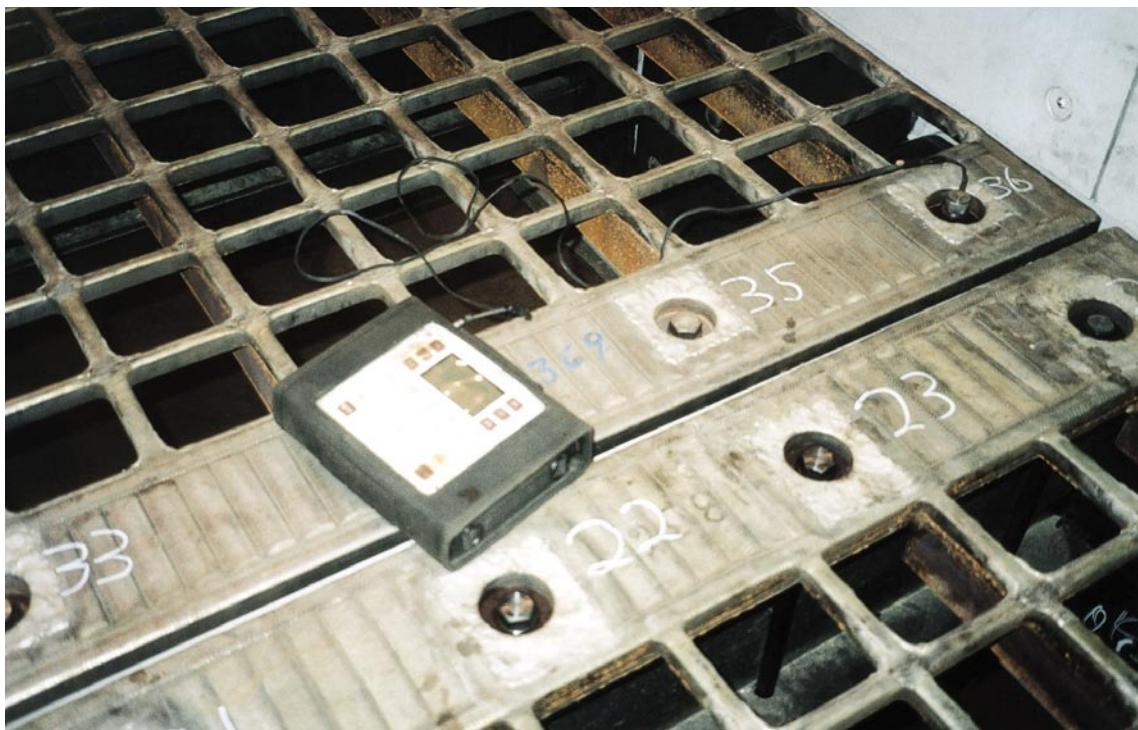
Special screens: highly corrosion-resistant and wide opened drilled plates coated with tungsten carbide
